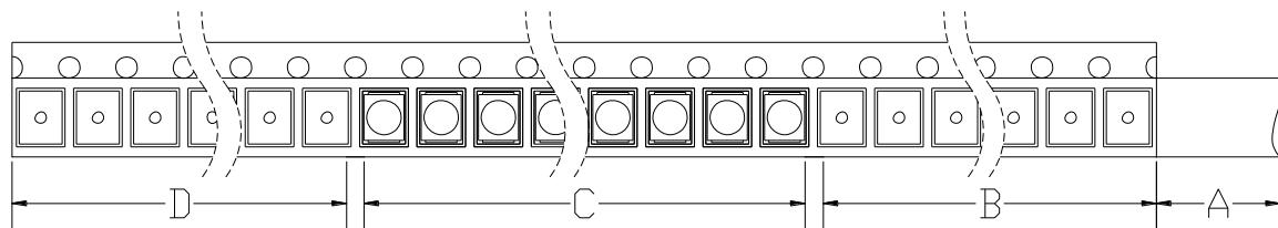
A: Top Cover Tape, 300mm; B: Leader, Empty, 200mm; C: 5000 Lamps Loaded; D: Trailer, Empty, 200mm.
